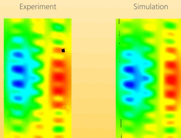
Figure 1 · Out-of-plane deformations of one tested POSICOSS panel
